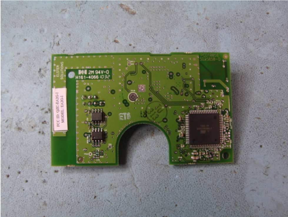
Figure 3: Location of Internal FCC Label on EA2G-I Printed Circuit Board Assembly
