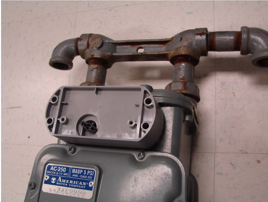
Figure 7: EA2G-I Module Partial Assembly – AMCO Gas Meter
