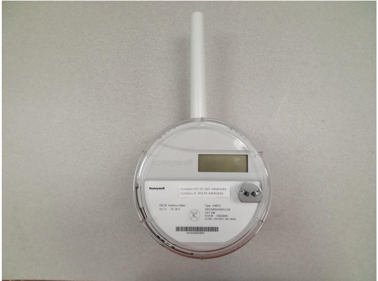
Label location on the front of A4 meter host
