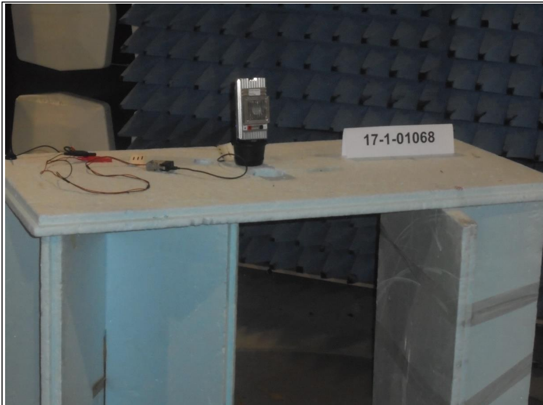
Photograph 3: Test set-up 3, EMI-field measurements
