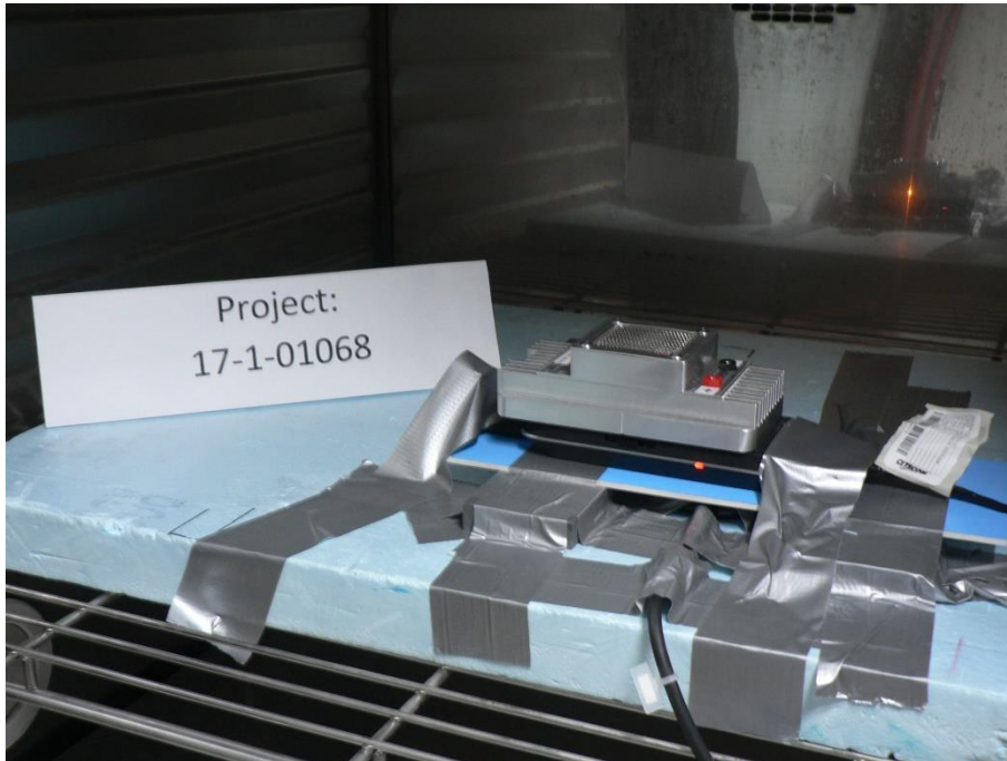
Photograph 5: Set-up for measurements on climatic chamber Tmin, Tmax
