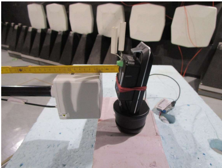
Photograph 6: Measurements in the anechoic chamber, 5cm distance between measurement probe and EUT, Position 5
