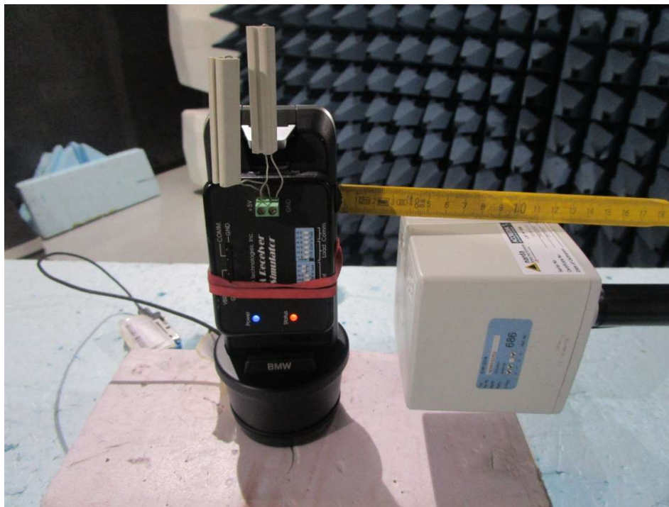
Photograph 2: Measurements in the anechoic chamber, 5 cm distance between measurement probe and EUT, Position 4
