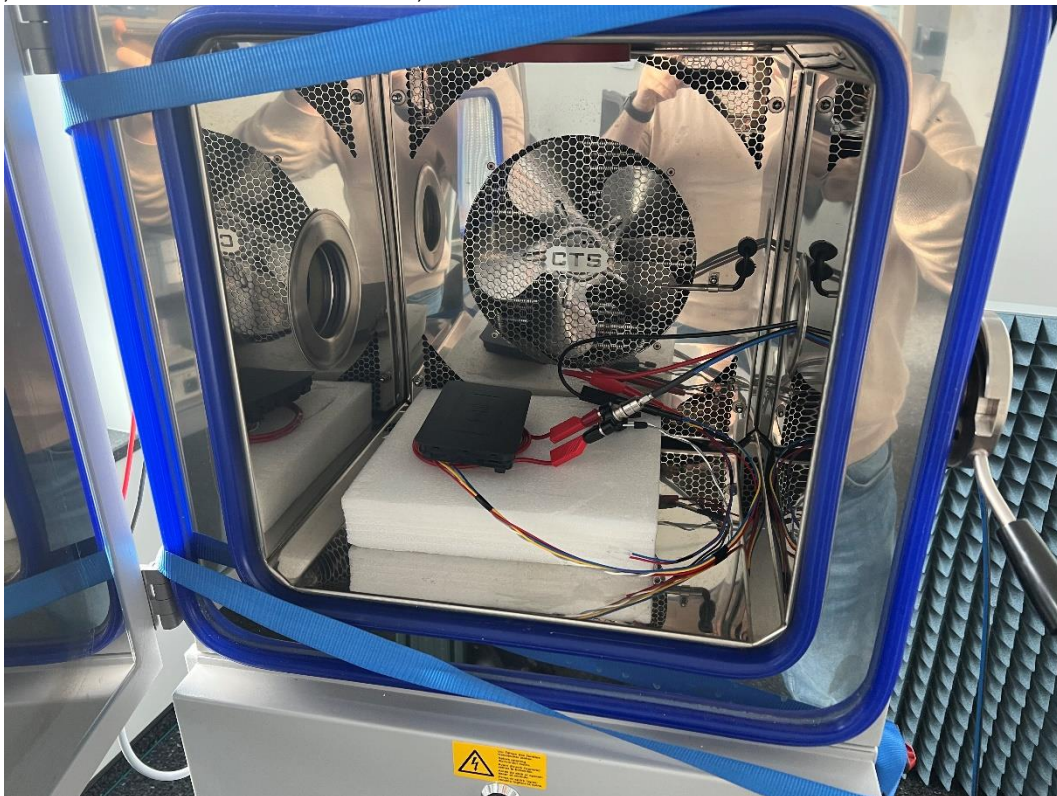
Photo No. 7, measurement in climatic chamber, overall view:
