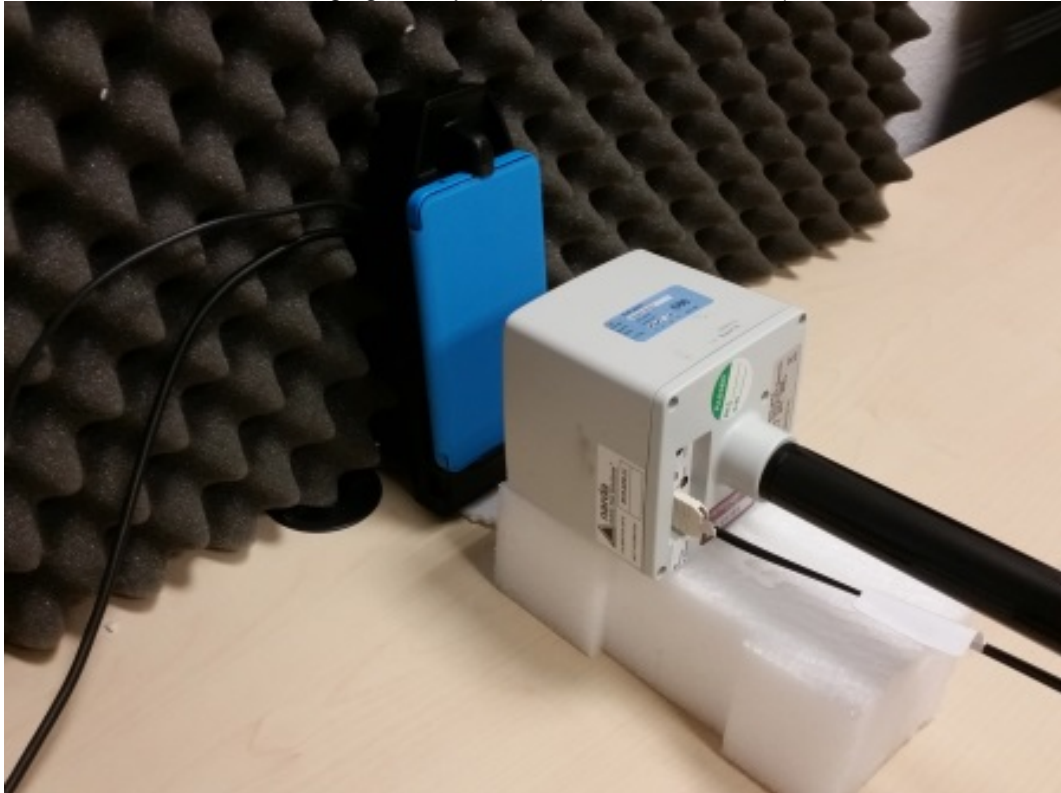
Photo 7: DUT - measurement position - left side with 10cm distance charging smartphone (Microsoft Lumia 640)
