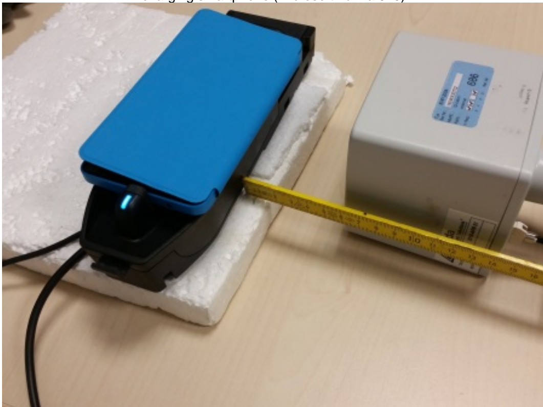
Photo 7: DUT - measurement position - left side with 10cm distance charging smartphone (Microsoft Lumia 640)
