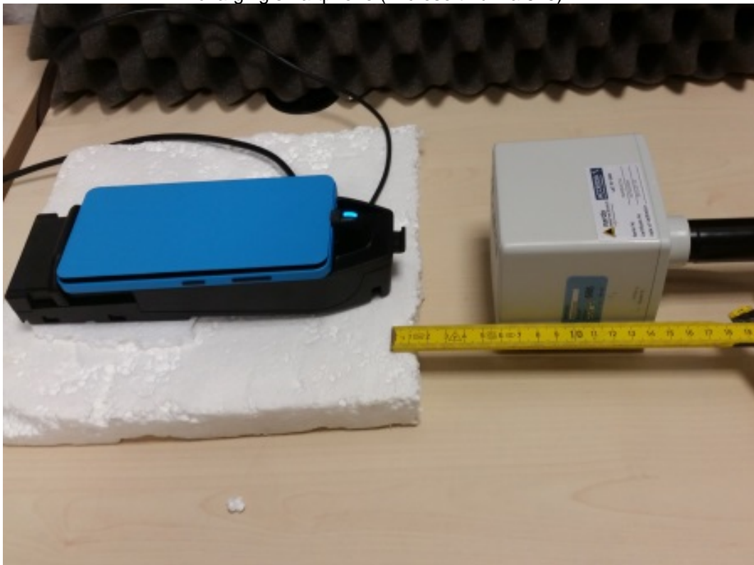
Photo 9: DUT - measurement position - front side with 10cm distance charging smartphone (Microsoft Lumia 640)
