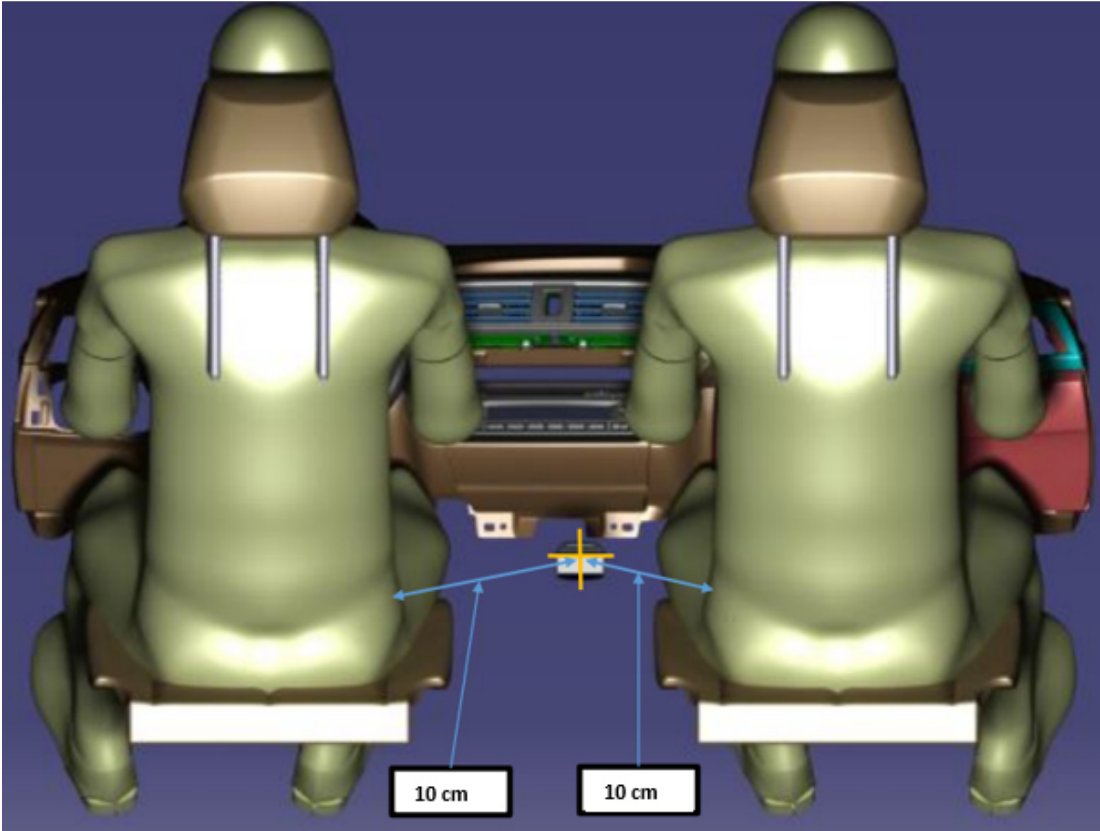
Diagram for the installation position with distances to human body
