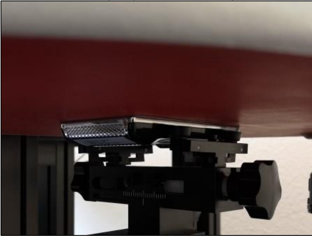
Photo 6: Test body worn position back side without any distance
