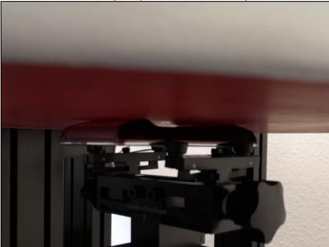
Photo 6: Test body worn position back side without any distance
