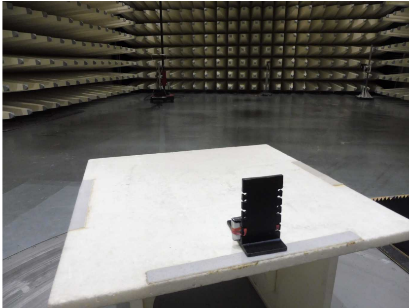
Photo 7: RSE set-up (30MHz to 1GHz)
