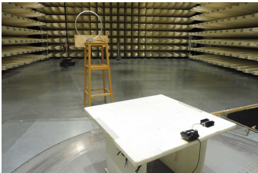
Photo 2: radiated emission with loop antenna, x-axis
