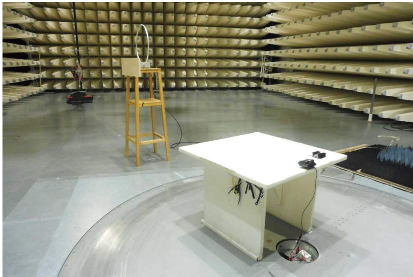
Photo 3: radiated emission with loop antenna, y-axis
