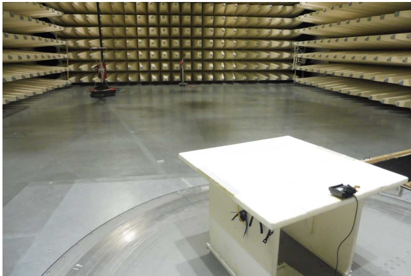
Photo 1: radiated emission < 1GHz
