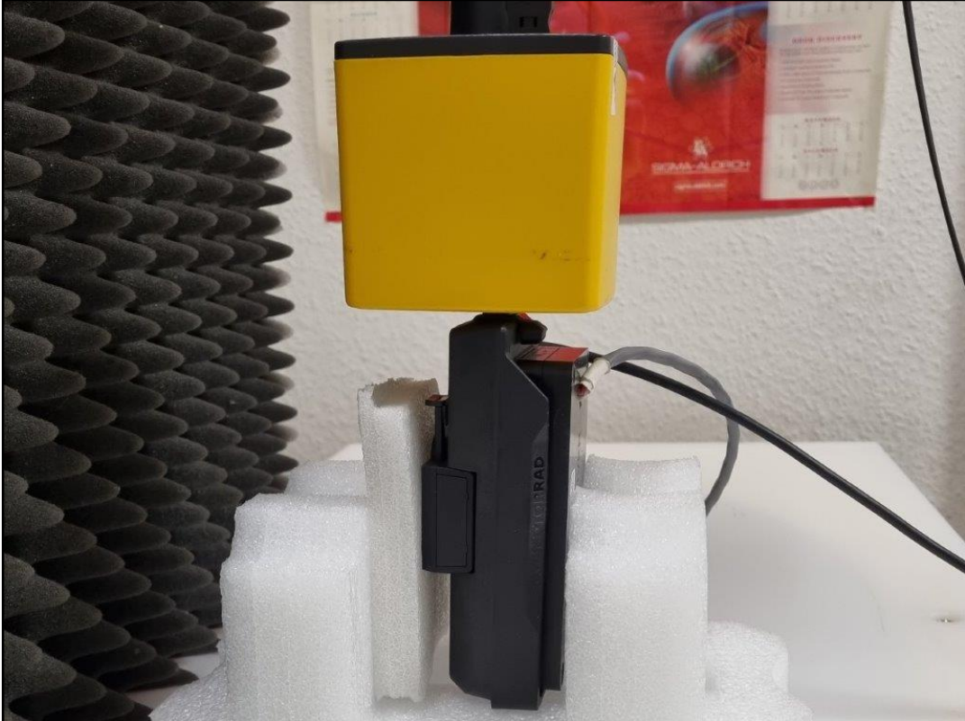
Photo 9: Test Position - Right side with 0cm to the centre of the probe (magnetic z-axis)
