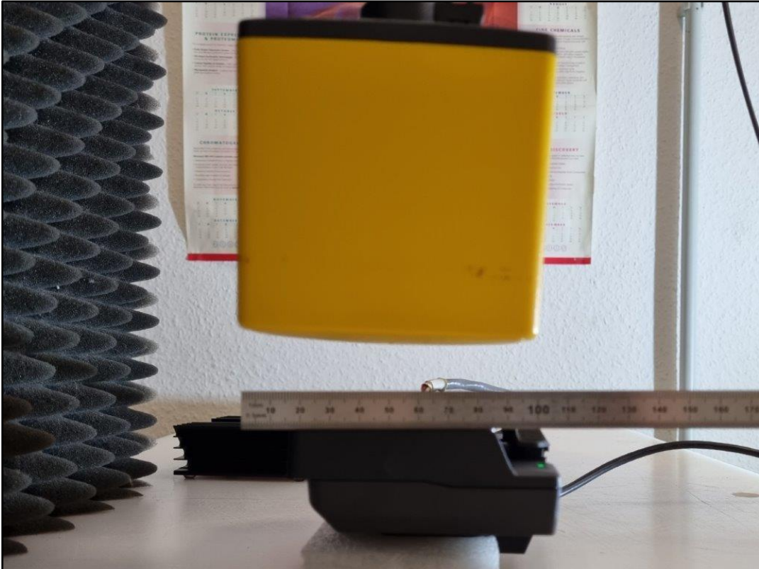
Photo 8: Test Position - Right side with 0cm to the centre of the probe (magnetic z-axis)
