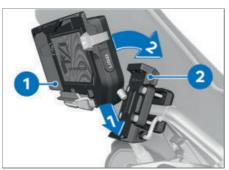
Slip the bottom edge of the Connected-Ride Cradle 1 into the lug of navigation preparation 2 and pivot the top edge forward. Make sure that the Connected-Ride Cradle is installed right way round.
