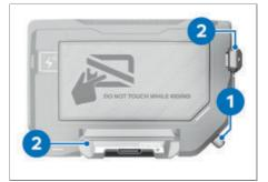
Slacken screw 1 and ease arms 2 far enough apart to slot the smartphone into the ConnectedRide Cradle.
