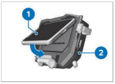
Insert the top edge of smartphone 1 into ConnectedRide Cradle 2. Make sure that the smartphone's charging socket is positioned on the right-hand side of the ConnectedRide Cradle.  Pivot the bottom edge of smartphone 1 down and insert it into Connected-Ride Cradle 2.
