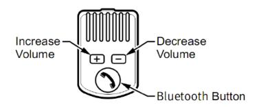
The microphone assembly consists of:
