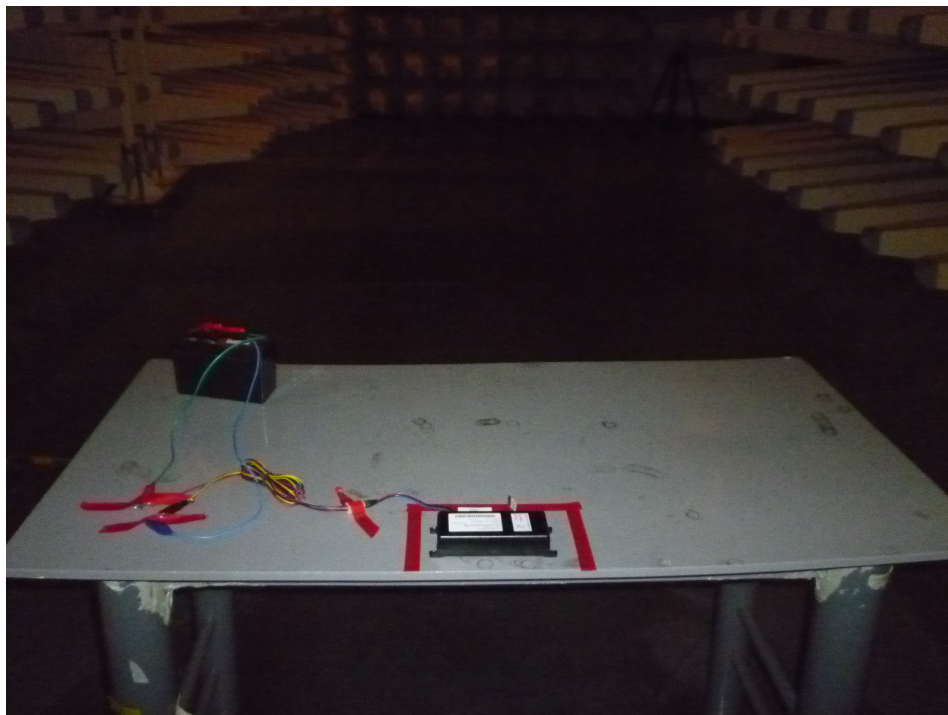
Setup for Radiated Emission
