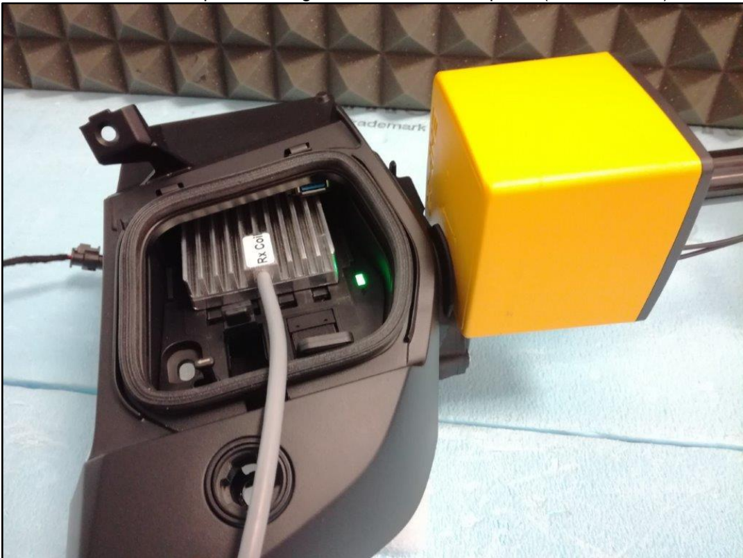
Photo 16: Test position - Right side with EHP 50F probe (0mm distance)
