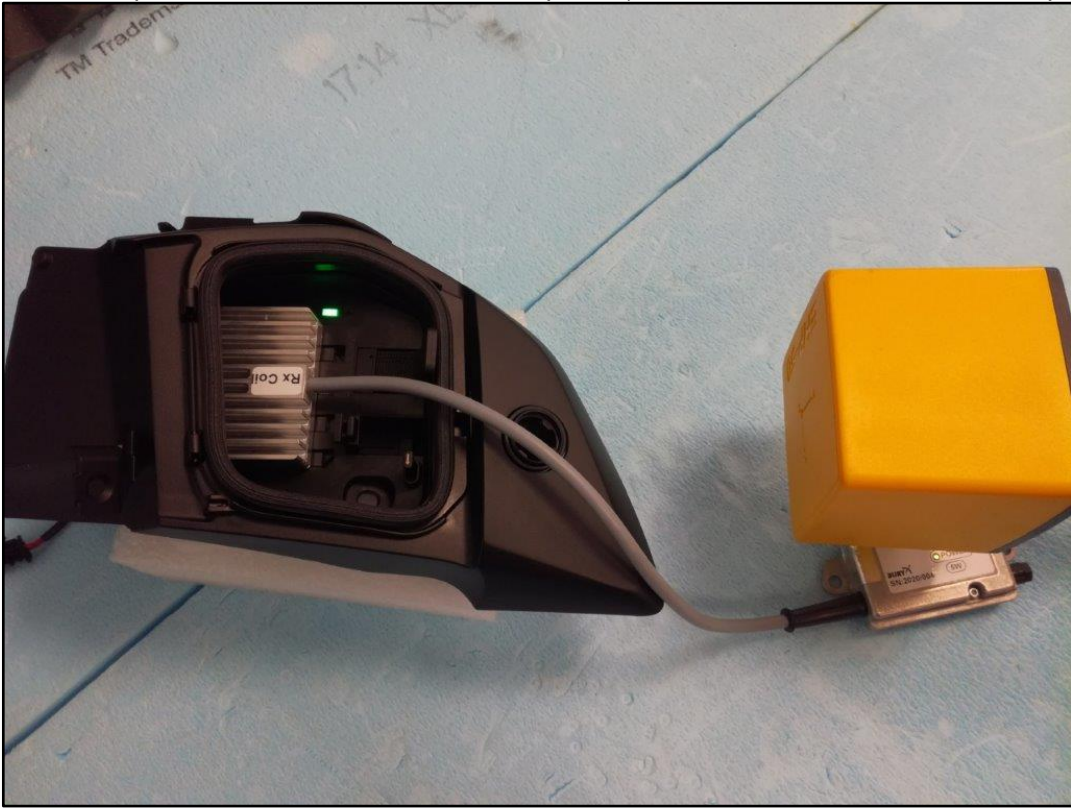
Photo 14: Test position - Left side with EHP 50F probe (0mm distance)
