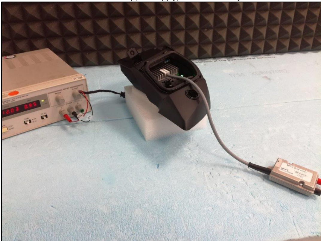
Photo 8: Test Setup, DC supply, DUT and dummy load
