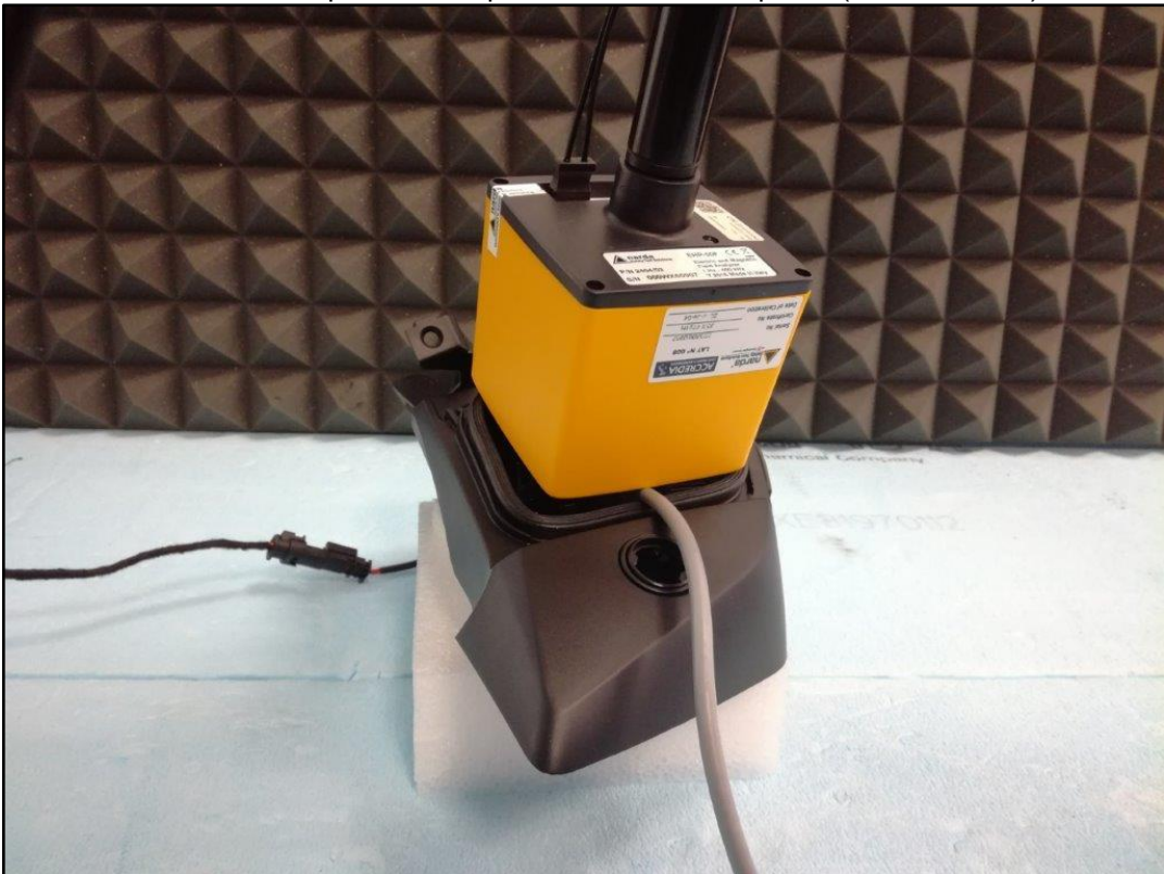
Photo 10: Test position - Top side with EHP 50F probe (0mm distance)
