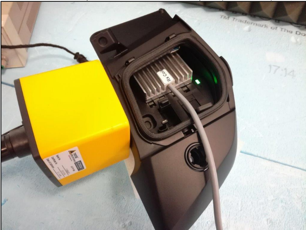
Photo 14: Test position - Left side with EHP 50F probe (0mm distance)
