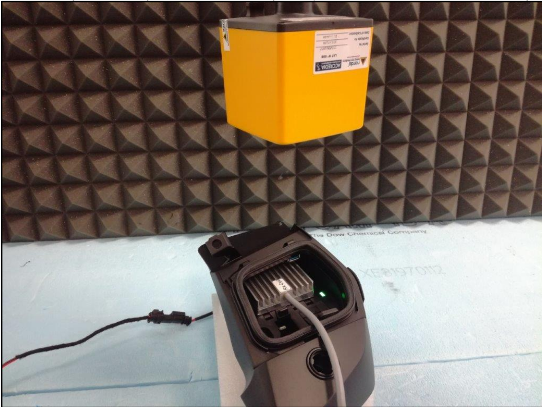
Photo 11: Test position - Top side with EHP 50F probe (20 cm distance to the centre of the probe)
