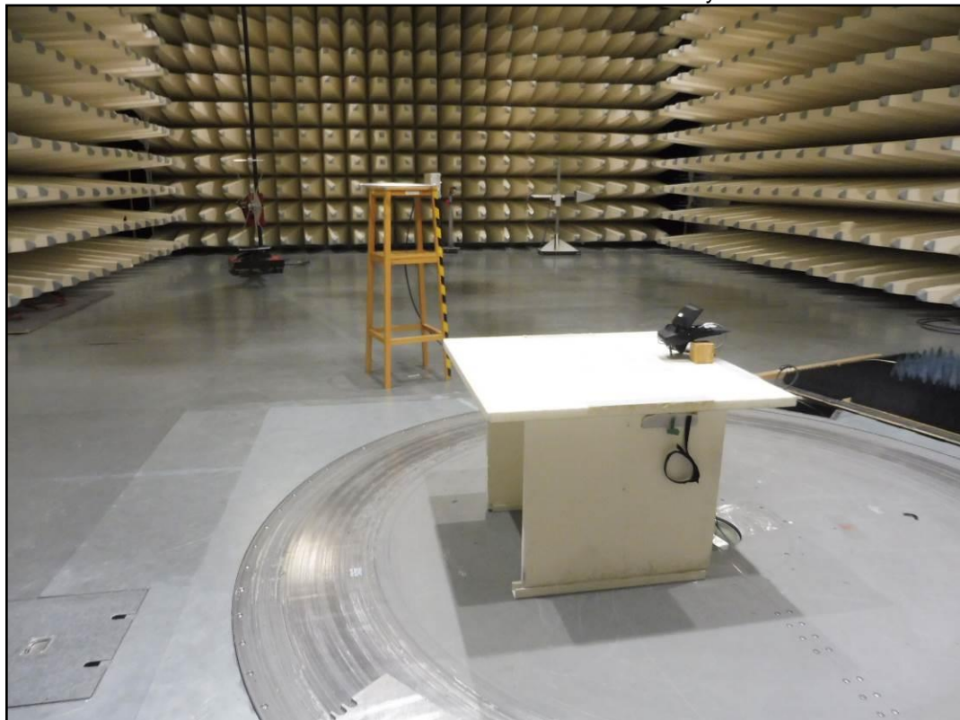
Photo 2: radiated emission 9KHz-30MHz set 1 y-axis
