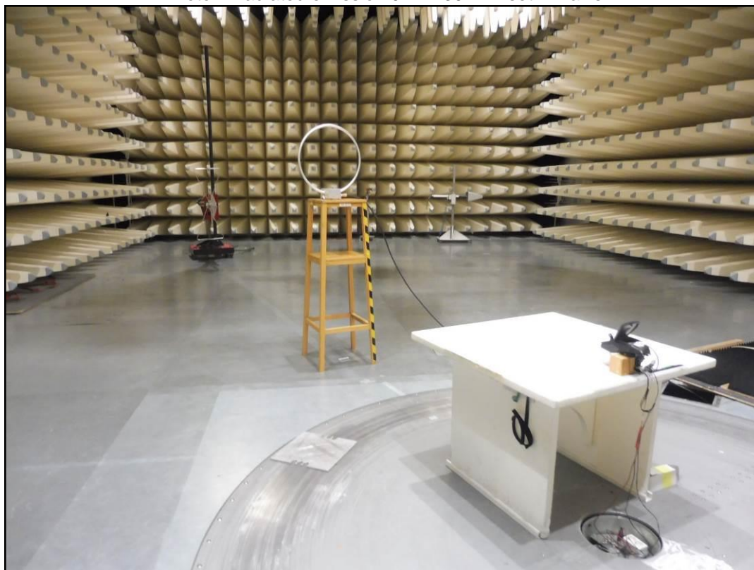
Photo 1: radiated emission 9KHz-30MHz set 1 x-axis
