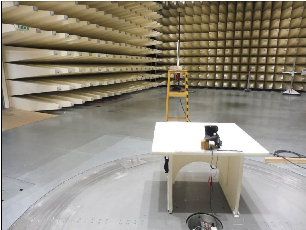
Photo 7: radiated emission 9KHz-30MHz z-axis set 2
