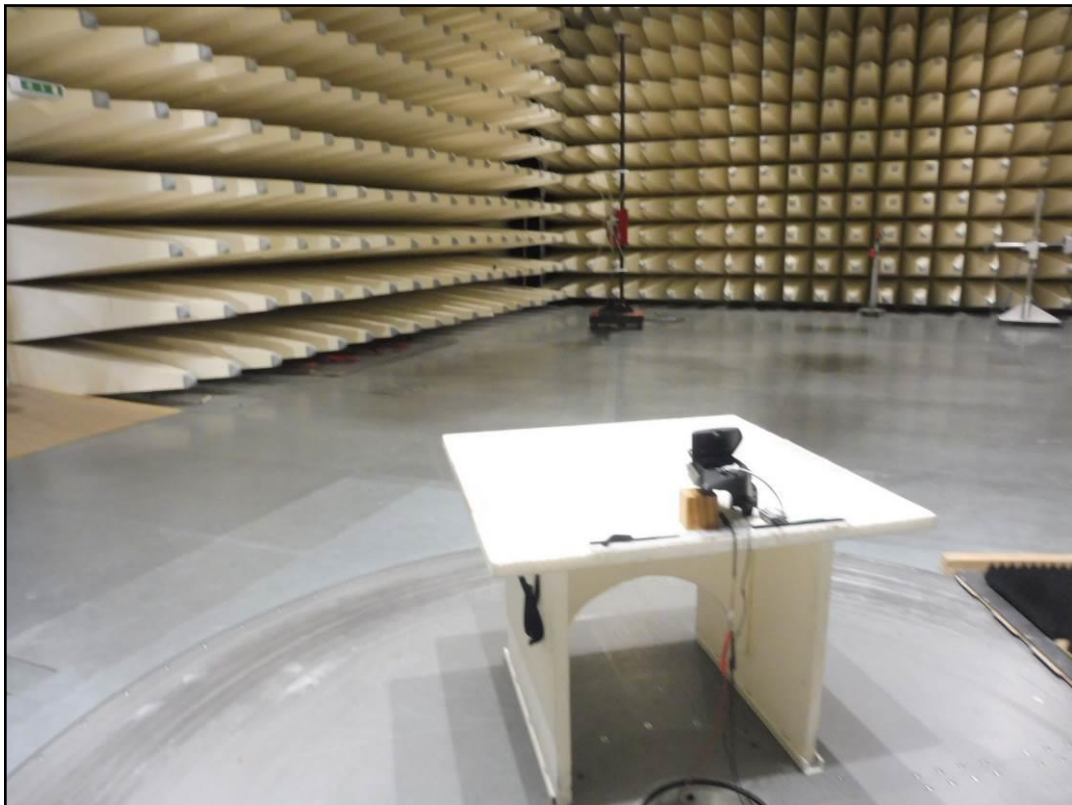
Photo 4: radiated emission 30MHz - 1GHz set 1
