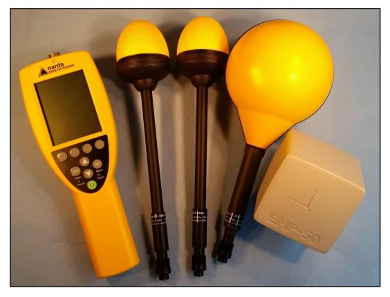
A state of the art Broadband Electromagnetic Field Test system was used. The probes of the system are fitted with three sensors which measure the field strength of the X, Y and Z plane directions separately. The field strength is calculated by the instrument's processor by summing the squares of the three measured values.
