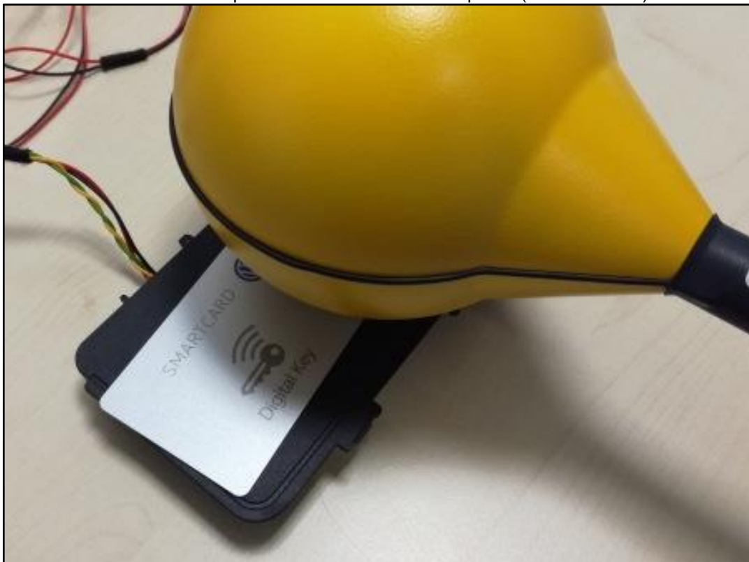
Photo 14: Test position - NFC with HF3061 probe (0mm distance)
