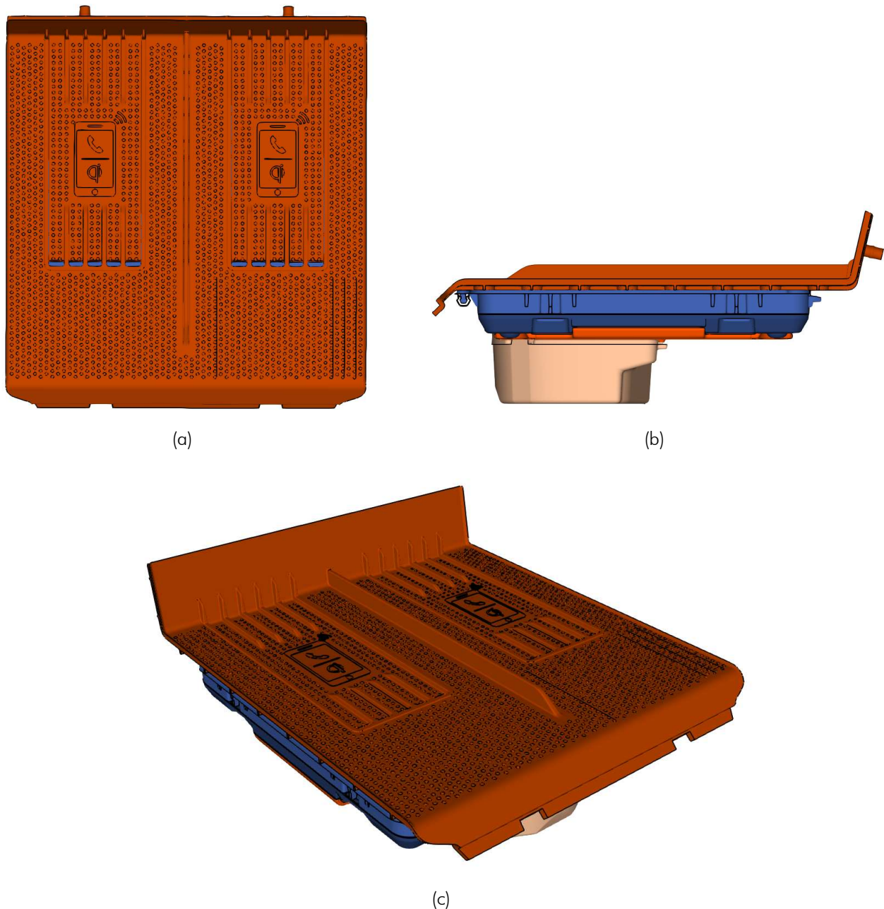
Figure 8: Geometry of the air grid (rubber mat) which was added on top of the DUT.
