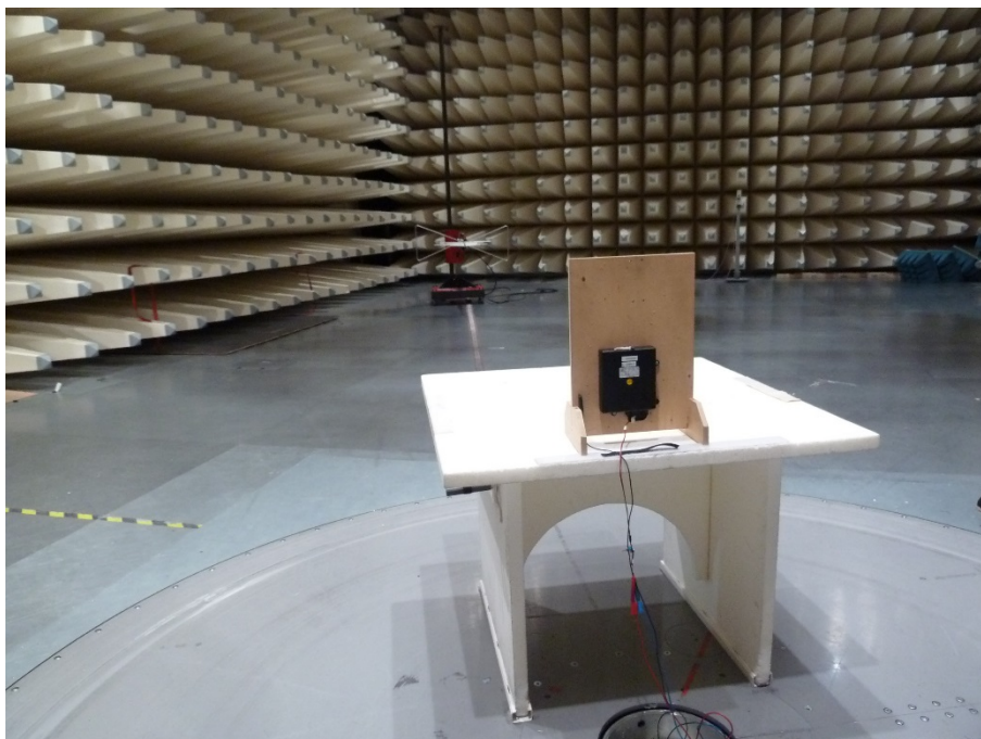
Photo 6: EUT at the semi anechoic chamber
