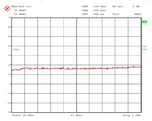
No significant frequencies above the noise floor of the system were found during the preliminary radiated emission test inside this frequency range, so no final measurements were carried out on the outdoor test site.
