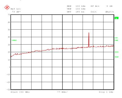
The following frequency was found outside the restricted bands during the preliminary radiated emission test:
