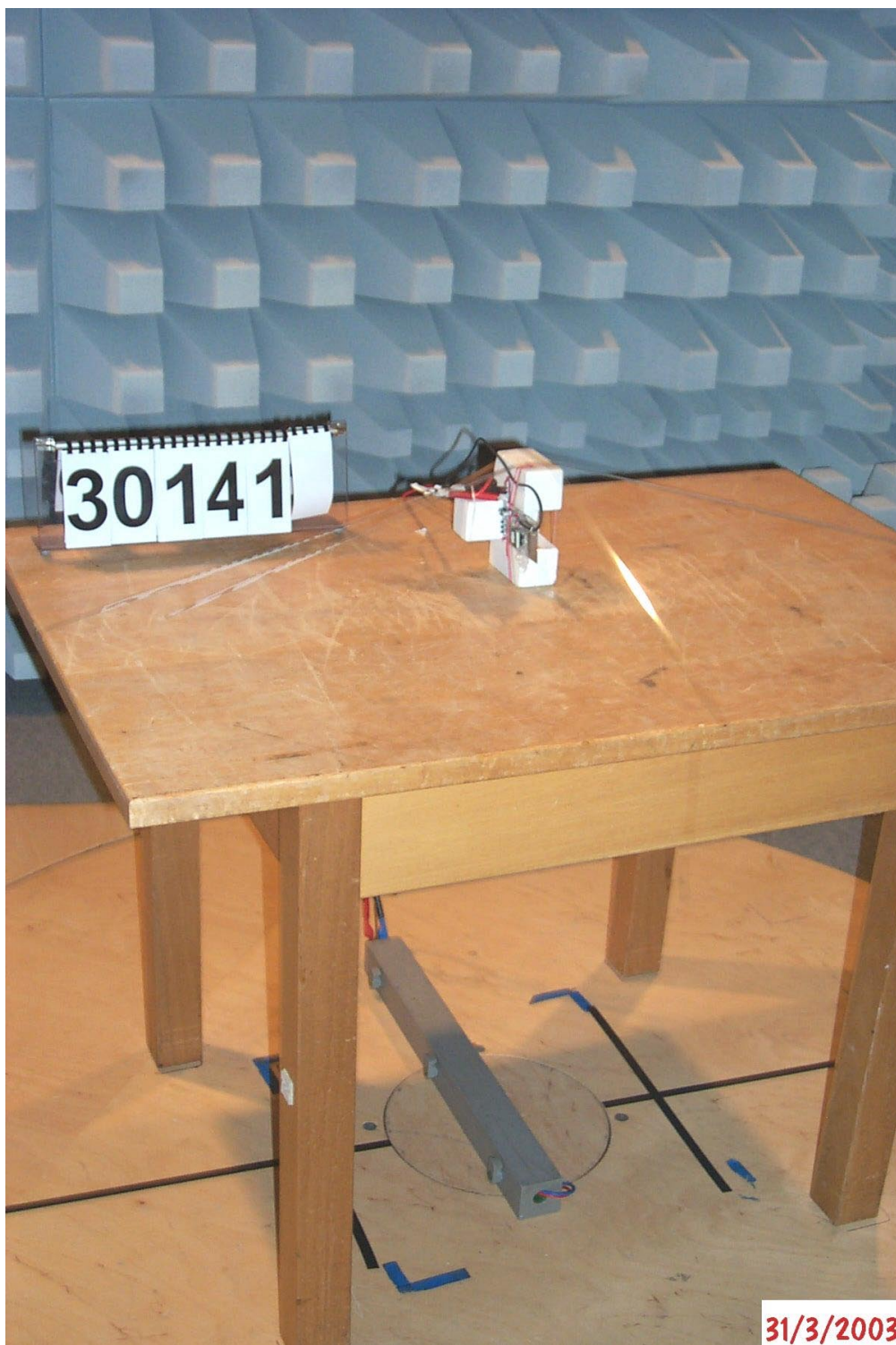
30141_a.jpg BCM001 test set-up preliminary emission test below 1 GHz
