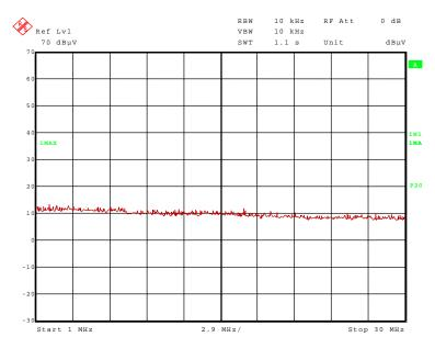
No significant frequencies above the noise floor of the system were found during the preliminary radiated emissions test, therefore no measurements were carried out on the outdoor test site.
