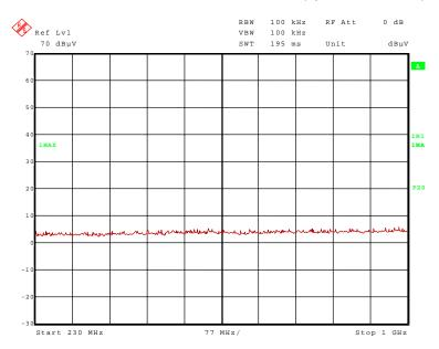
No significant frequencies above the noise floor of the system were found during the preliminary radiated emission test inside this frequency range, so no measurements were carried out on the open area test site.
