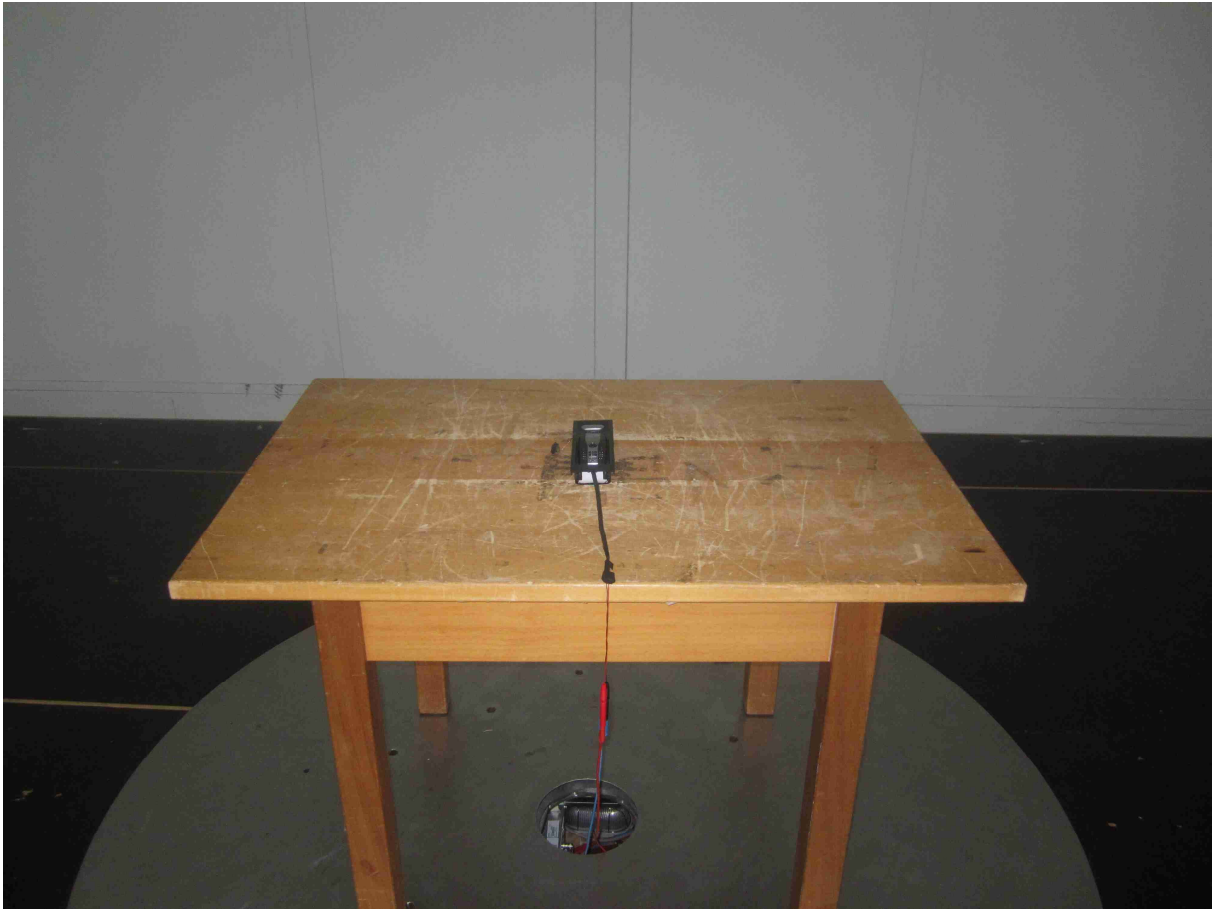
122097_04: Test setup - Radiated emission – 30 MHz – 1 GHz (open area test site)
