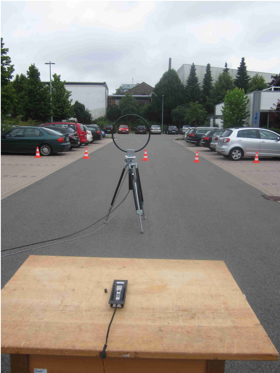
122097_06: Test setup - Radiated emission – 30 MHz – 1 GHz (outdoor test site)
