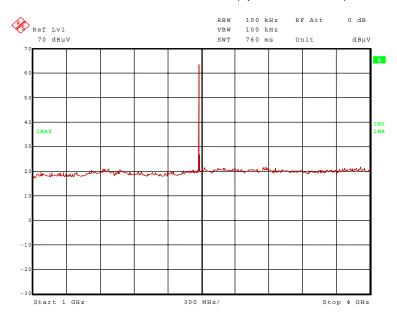
122097 41.wmf: Spurious emissions from 1 GHz to 4 GHz (operation mode 3):
