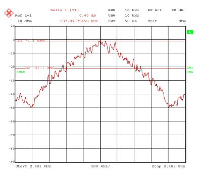
122097 49.wmf: 20 dB bandwidth at the middle of the assigned frequency band (mode 2):
