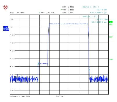
122097\_30.wmf: Dwell time at the middle of the assigned frequency band (operation mode 2a):
