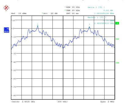
122097\_26.wmf: Channel separation at the middle of the assigned frequency band (mode 2):
