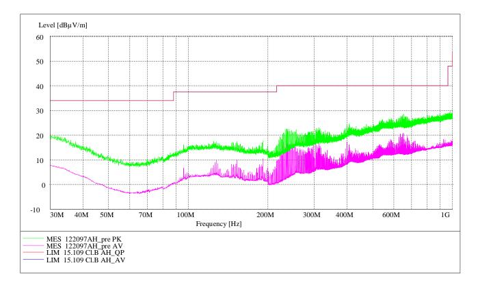
The following frequencies were found during the preliminary radiated emission test:
