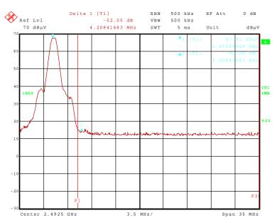
122097\_07.wmf: Radiated band-edge compliance, upper band edge, hopping off (mode 3):
