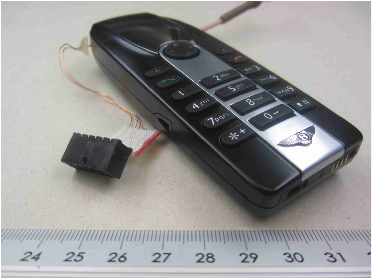
122097_60.JPG: EUT – handset, with temporary antenna connector, 3D top view* 2
