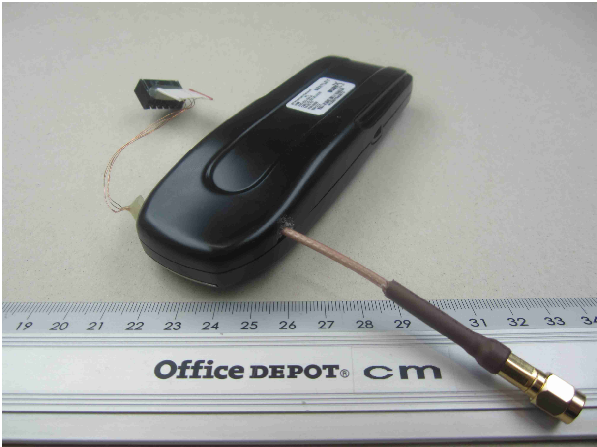
122097_61.JPG: EUT – handset, with temporary antenna connector, 3D bottom view* 2
