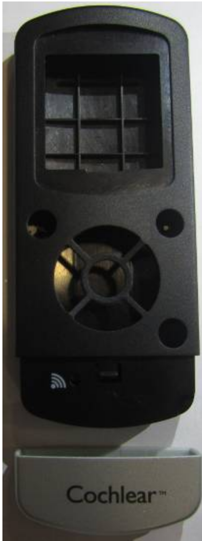
Front, bottom cover removed (symbol for pairing button) (no display and buttons)
