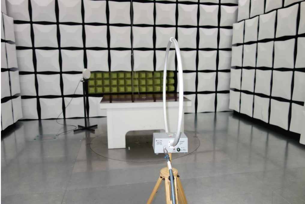
Picture 1: Loop Antenna Parallel to Axis
