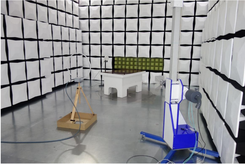
Picture 5: Loop Antenna Perpendicular to Axis
