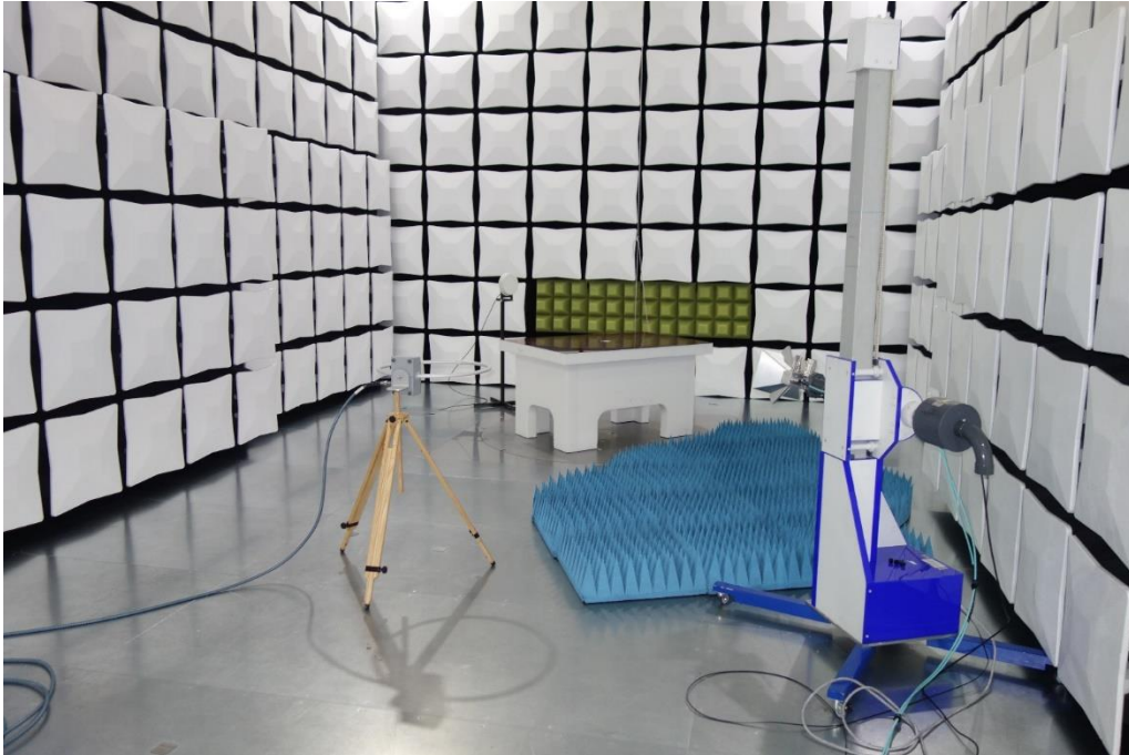
Picture 3: Loop Antenna Parallel to Floor
