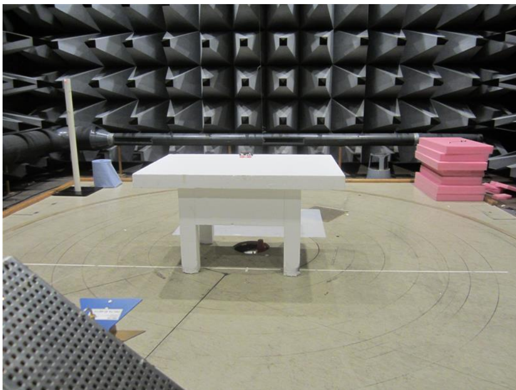
Photo 4.10.1 Test setup regarding measurement of field strength of fundamental.
