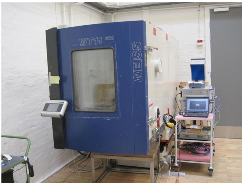
Photo 4.6.1 Test setup regarding measurement of 20 dB bandwidth.
