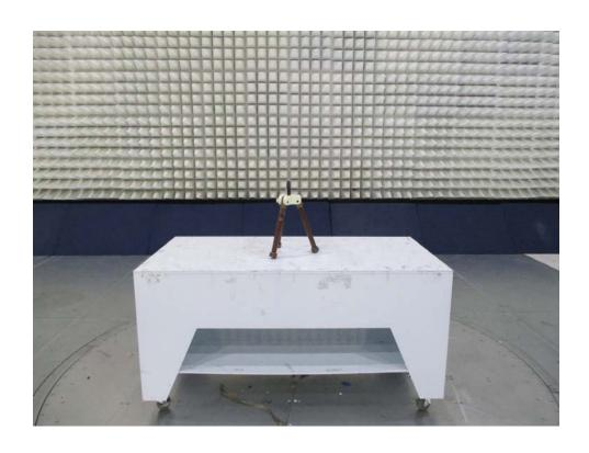
Radiated Emissions Transmitting mode Horizontal location of the EUT
