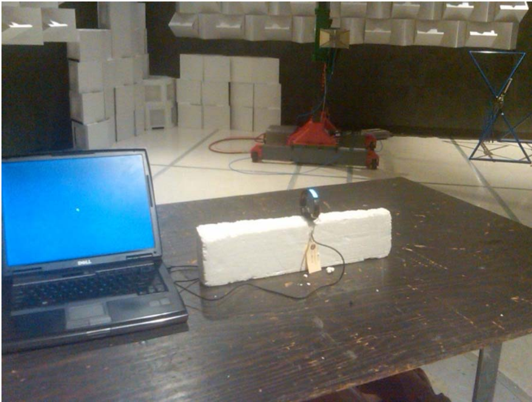
Test Setup – Radiated Emissions (above 1 GHz)
