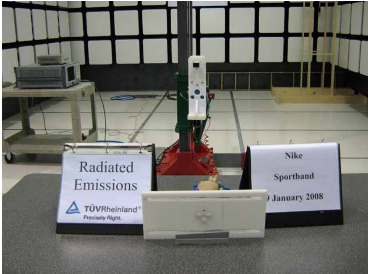
Test Setup: Radiated Emission from 18GHz to 26GHz at 1 Meter Distance – Rear View
