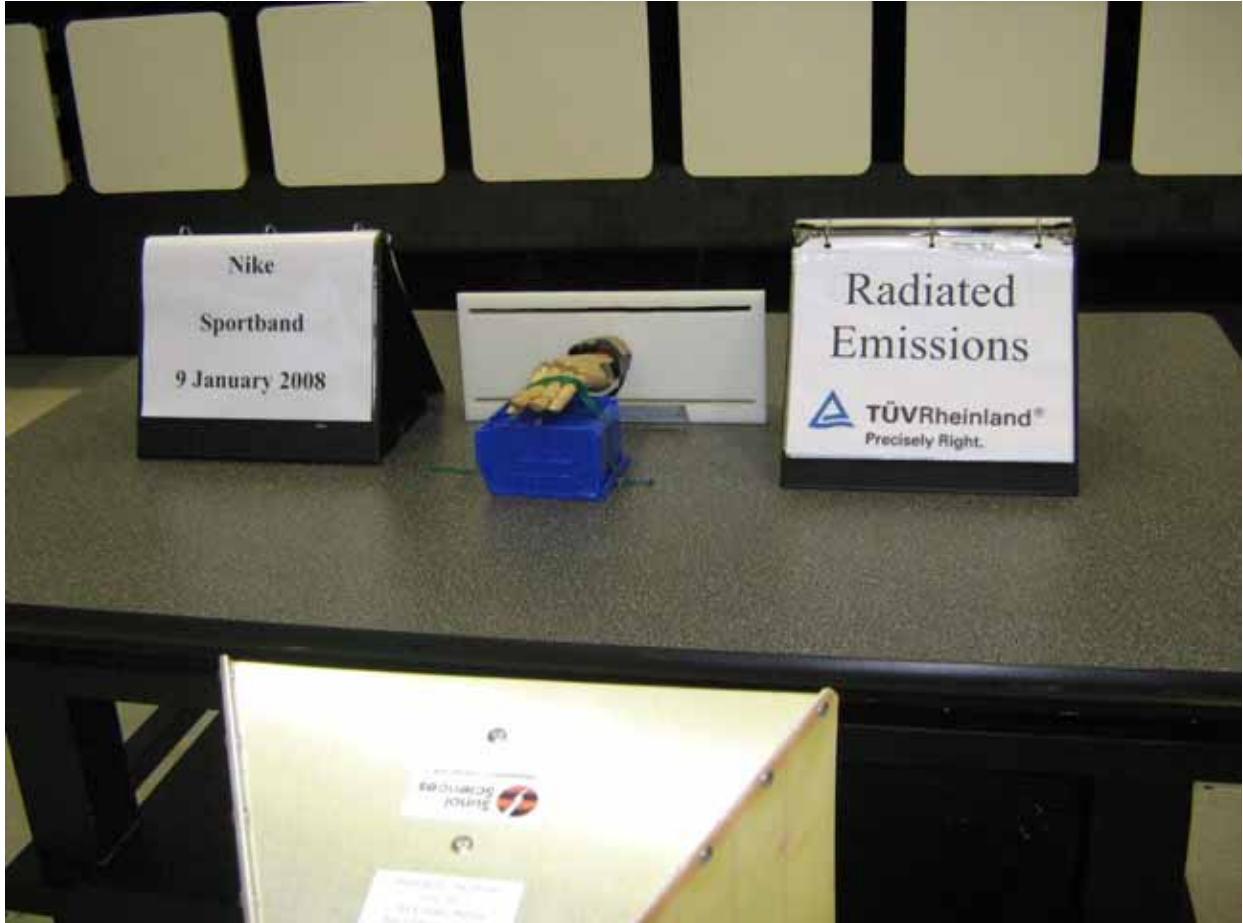
Test Setup: Radiated Emission from 6.5GHz to 18GHz at 1 Meter Distance – Front View
