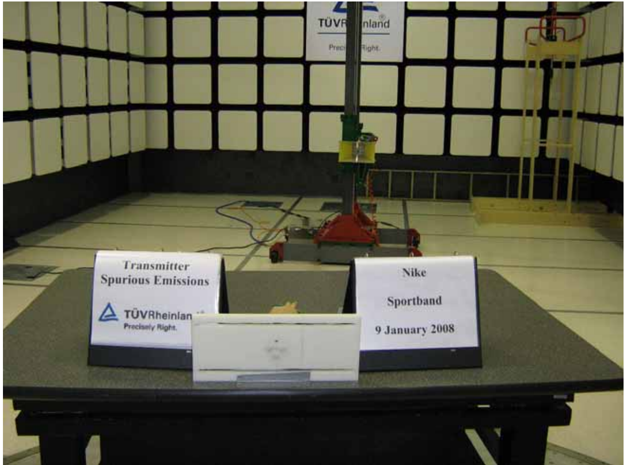
Test Setup: Radiated Emission from 1GHz to 6.5 at 3 Meter Distance – Rear View
