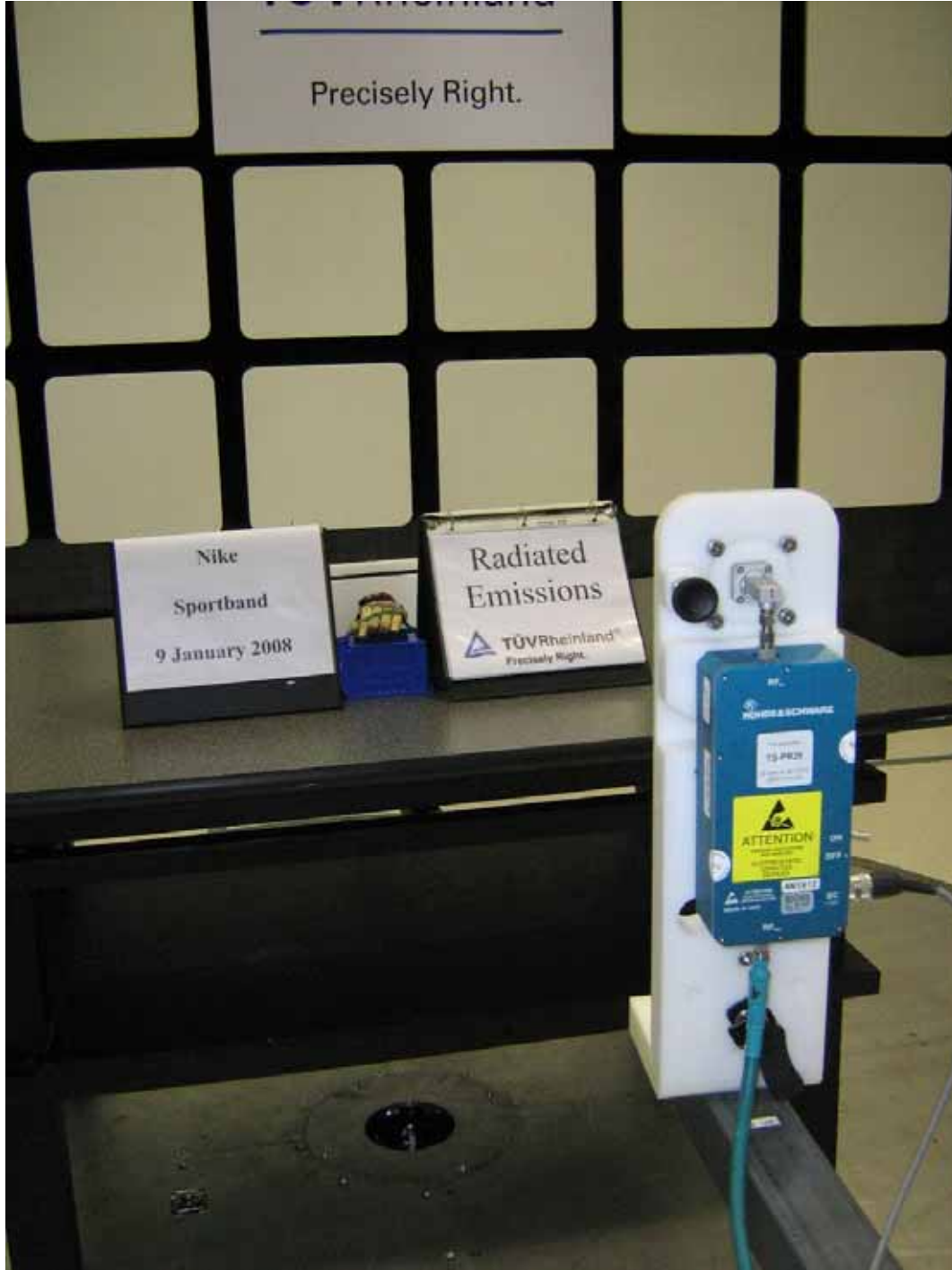
Test Setup: Radiated Emission from 18GHz to 26GHz at 1 Meter Distance – Front View
