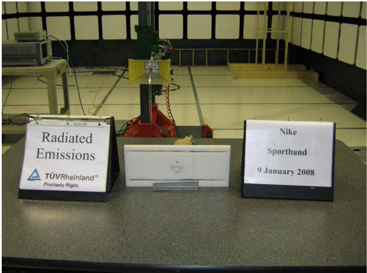
Test Setup: Radiated Emission from 6.5GHz to 18GHz at 1 Meter Distance – Rear View
