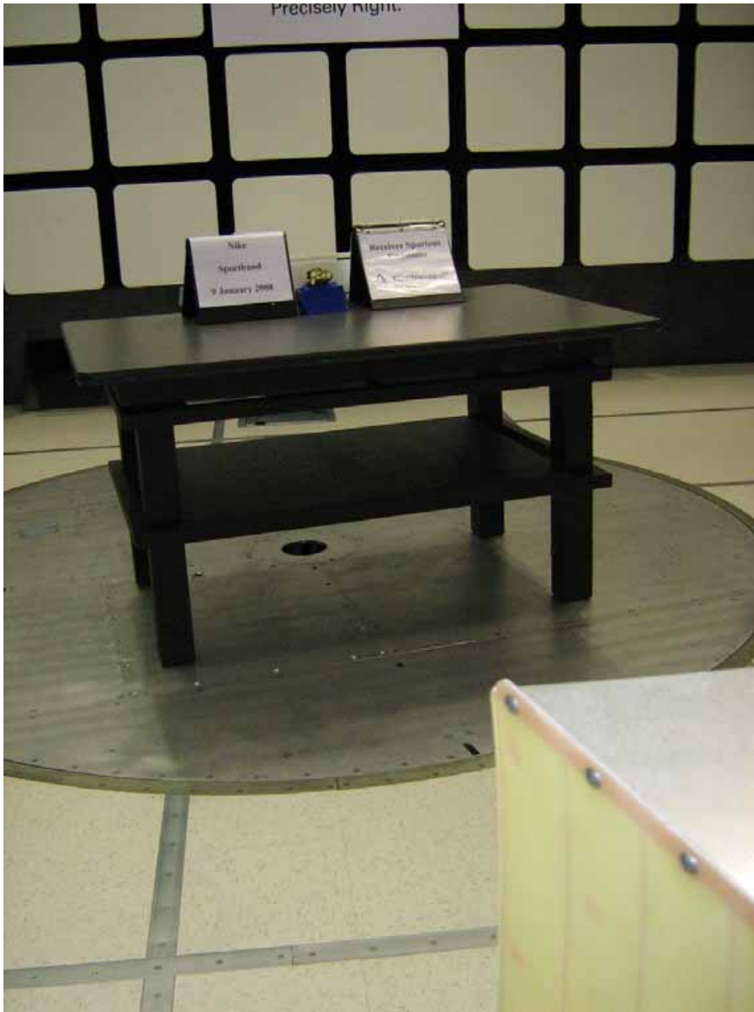
Test Setup: Radiated Emission from 1GHz to 6.5 at 3 Meter Distance – Front View
