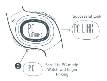
**NOTE:** The link has failed if the display reads **PC NOT FOUND**. Press **START** to retry.
