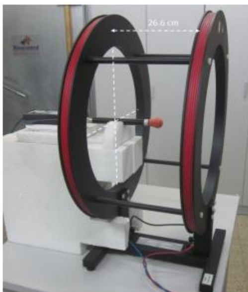
Figure 2: Calibration set-up in the Helmholtz coils system – B field
