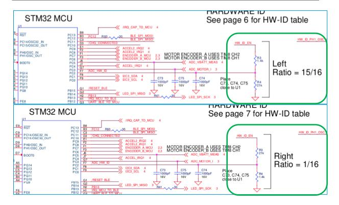
Resistance is switched (1.4K / 21K left engine, 21k / 1.4k right engine) Differences:
