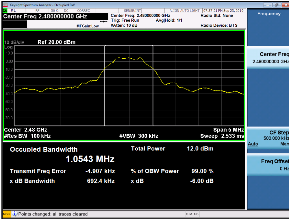
6 dB Bandwidth plot (High-CH 39)
