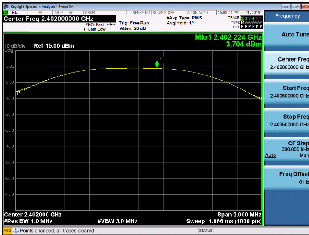
Conducted Output Power (Mid-CH 19)
