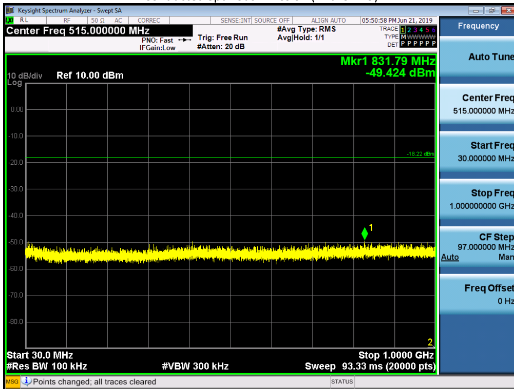
Conducted Spurious Emission (Mid-CH 19)
