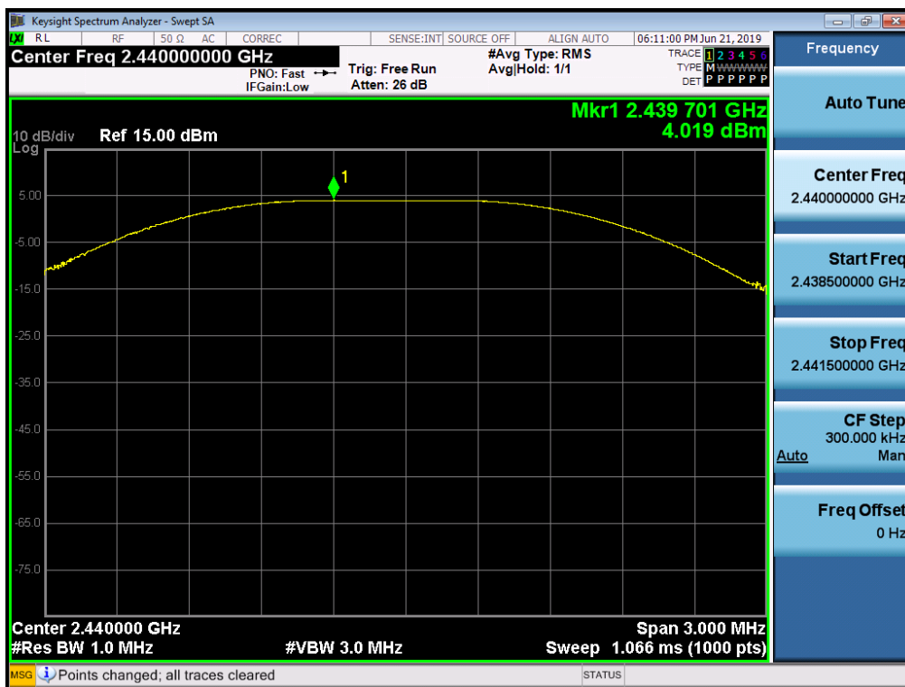
Conducted Output Power (Mid-CH 19)
