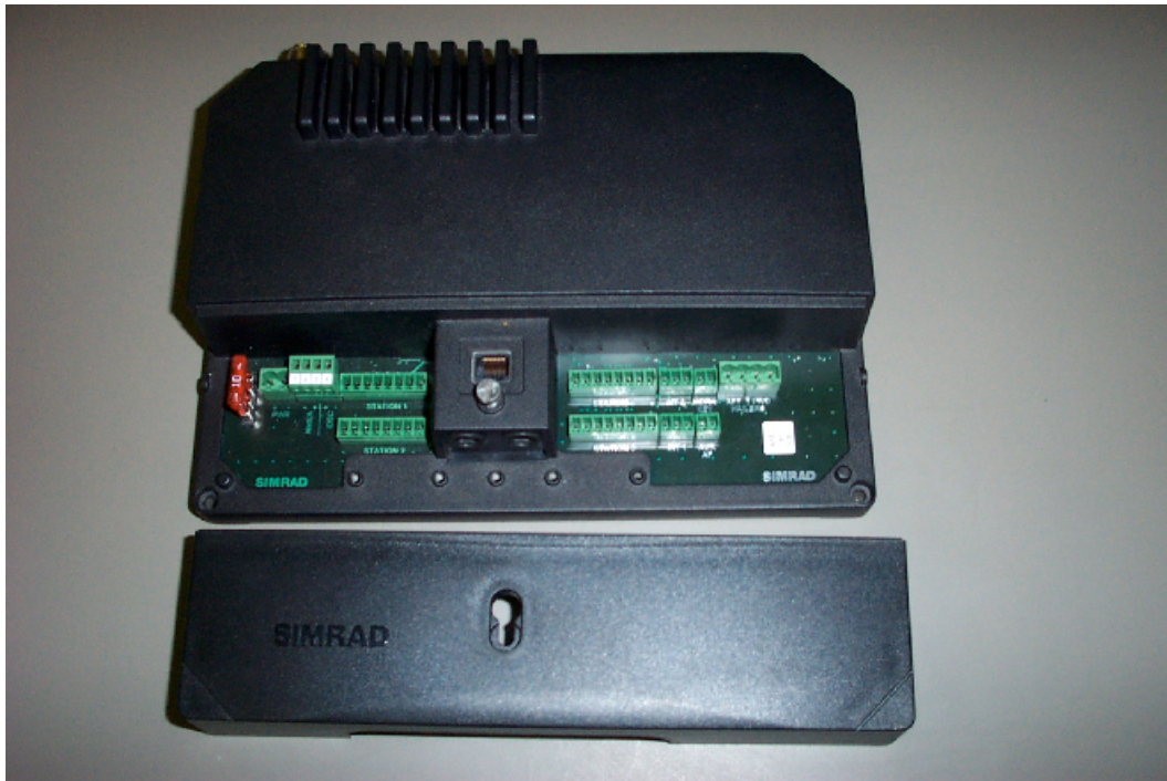
Fig 2: External view of transceiver unit, showing connectors
