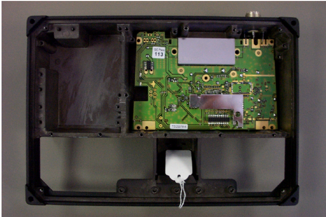
Fig 3: Interior View of Transceiver showing RF PCB only
