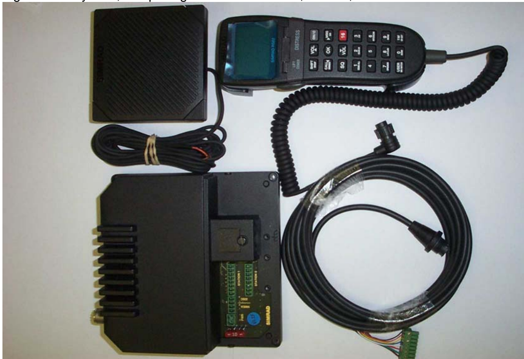
Fig 2: RS82 system, comprising RS80B transceiver, AHS82, LS80 and EXAH05 cable
