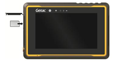
NOTE: To remove the SIM card, slightly push in the card to release it and then pull the card out of the slot.
