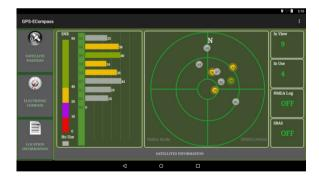
SBAS (satellite-based augmentation system) provides additional accuracy and reliability for the GPS devices. Ground stations are necessary to achieve the purpose. The SBAS feature works where such stations exist. You can enable the SBAS feature. (See "
