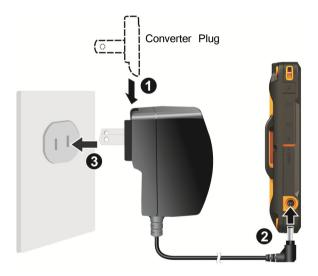
The charge indicator glows in amber when charging is in progress. Do not disconnect your device from AC power until the battery is fully charged, as indicated by the amber indicator turning into green. This will take a couple of hours.
