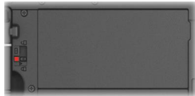
Incorrect (revealing red part)
