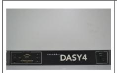
The DASY4/DASY5 measurement server is based on a PC/104 CPU board with a 166MHz low-power Pentium, 32MB chip disk and 64MB RAM. The necessary circuits for communication with either the DAE3 electronic box as well as the 16-bit AD-converter system for optical detection and digital I/O interface are contained on the DASY4/DASY5 I/O-board, which is directly connected to the PC/104 bus of the CPU
