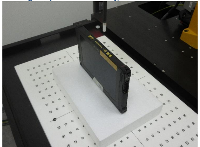
Testing Setup for Power Density, Bottom Side at 0 mm
