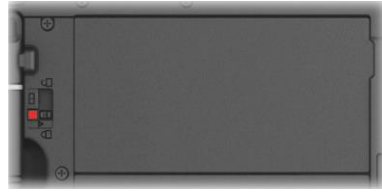
Incorrect (revealing red part)
